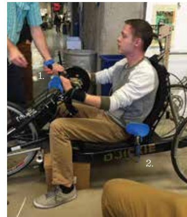
Matt Parkin (B.S. Design '15) 1. Adaptive pedal for cyclists with spinal cord injuries.
