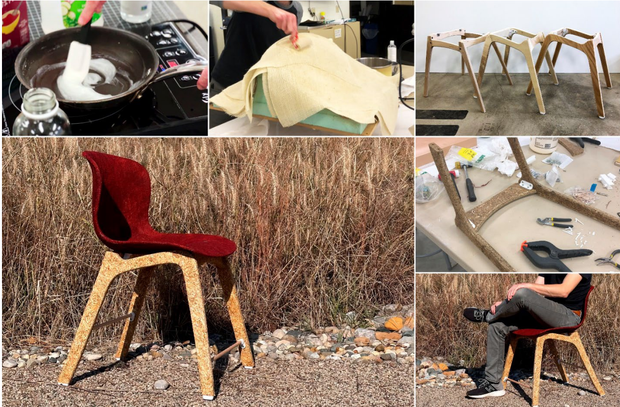
Figure 2. Build Process; Clockwise from top left: Adhesive Preparation, Seat Lamination, Structure Samples, Prototype Construction, The Fiber Chair v1 (Madder Root Dyed Jute Textile, Recycled Fabric, Straw, Plant Starch, PLA, Metal Fasteners). Photographs.
