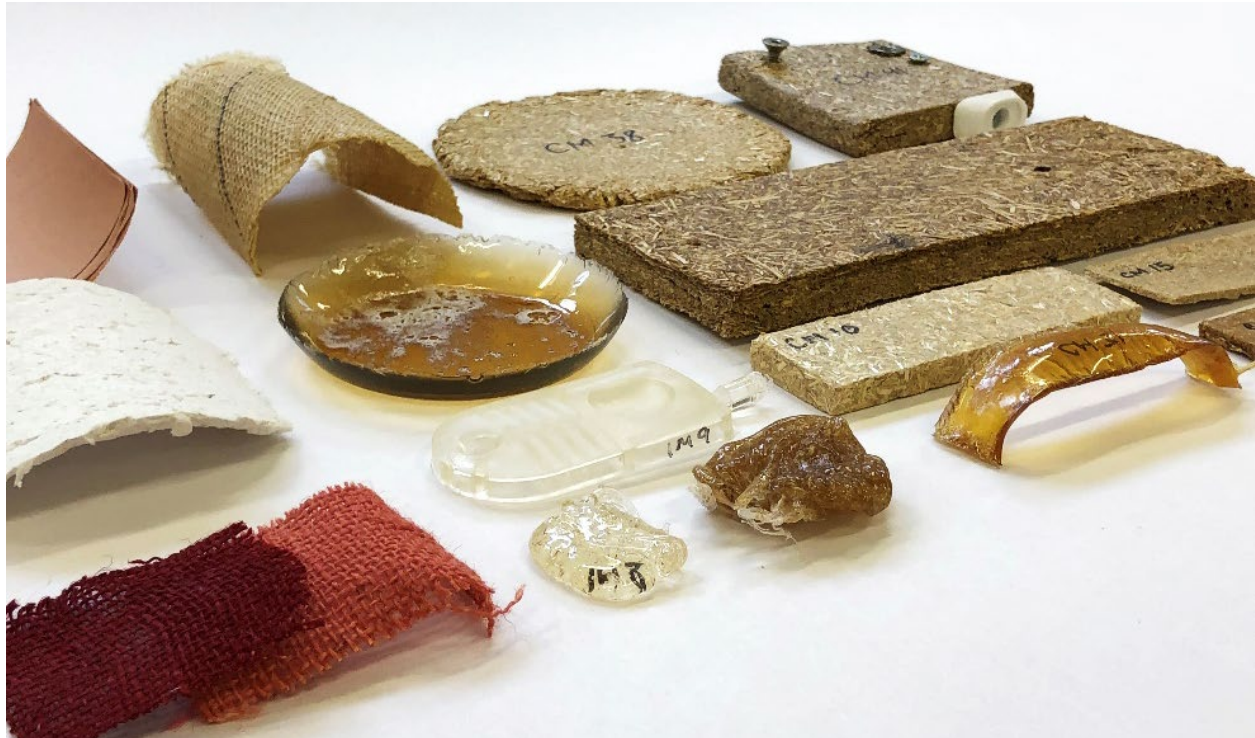
Figure 1. Bio-composite Samples. Jute Textile, Straw, Plant Starch, Rice Starch, Gelatin, Sugarcane, Paper, Madder Root. Photograph.
