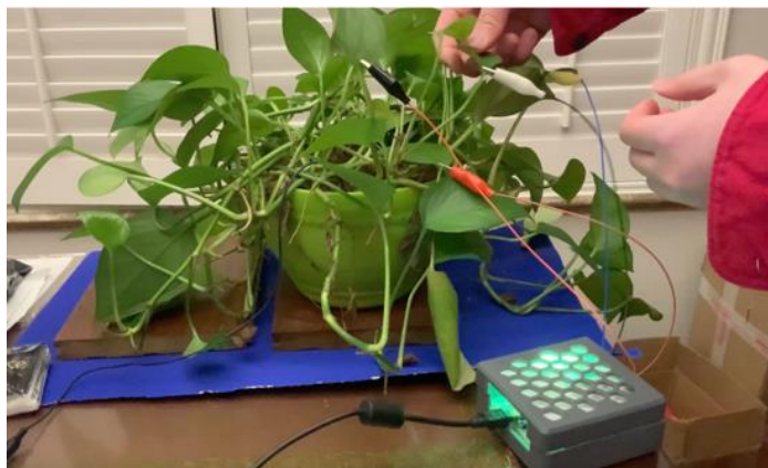
Figure 2. Display of PlantMIDI. The plant depicted in the image is a soil-grown Pothos plant. The product incorporates the use of a WS2812B LED strip, specifically chosen in green color (RGB:0,255,0) to enhance the aesthetic appeal and resemble plants. The casing is made from resin material and it is 3D printed.
