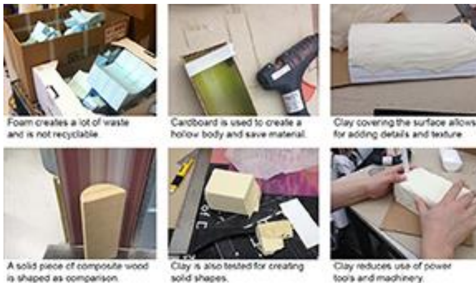
Figure 4. Testing of more environmentally friendly materials for model making.
