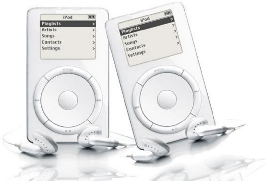
Figure 1. The Apple iPod was designed so that only an electronic specialist could replace a broken battery. This led users to throw away many, possibly the majority, of these circuit laden devices before it was necessary. Like all systems that were designed for obsolescence, this product may have boosted sales, but it unnecessarily created pollution and wasted an immense amount of resources.
