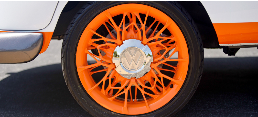
This VW wheel was redesigned and is 18% lighter. Read More > Image courtesy of Volkswagen.
