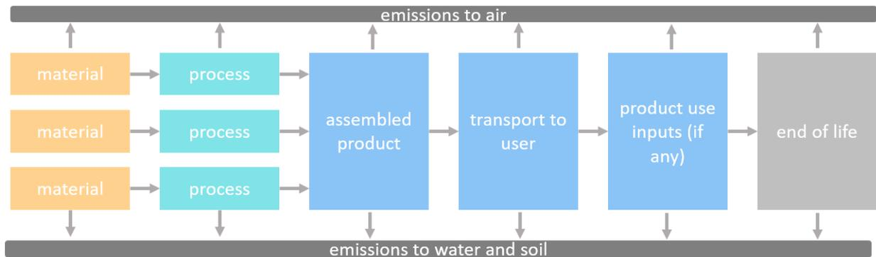
Figure 1. Impact points were calculated for each stage of the cradle to grave process. In the baseline product example, end of life was set to landfill which corresponds to the region's protocols for small electrical products.
