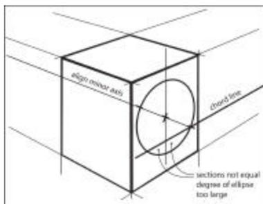
In the image to the right shows the degree of the ellipse is too small. The section to the right of the horizontal line is smaller than the section to the left. In both images the minor axis orientation is aligned with the left vanishing point and the chord line is drawn to the right vanishing
