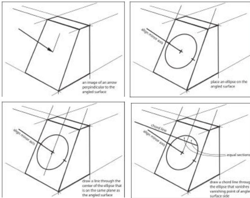
Draw a line that appears to be visually perpendicular with the angled surface. Draw an ellipse with the minor axis aligned with the perpendicular line. Draw another line through the center of the ellipse that is on the same plane as the angled surface. Next, draw a chord line at the top of the ellipse, which vanishes in the same direction as the angled surface. This lines should intersect the line that is drawn
