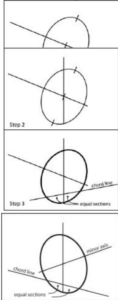
The following examples show ellipses that are not correct. As you can see the two sections created by the chord line are not equal. In the first image the ellipse is too large; the degree of the ellipse is large. Remember, the size of the ellipse is determined by the major axis and the degree is determined by the minor axis. Here, the minor axis distance, the degree, is too large.
