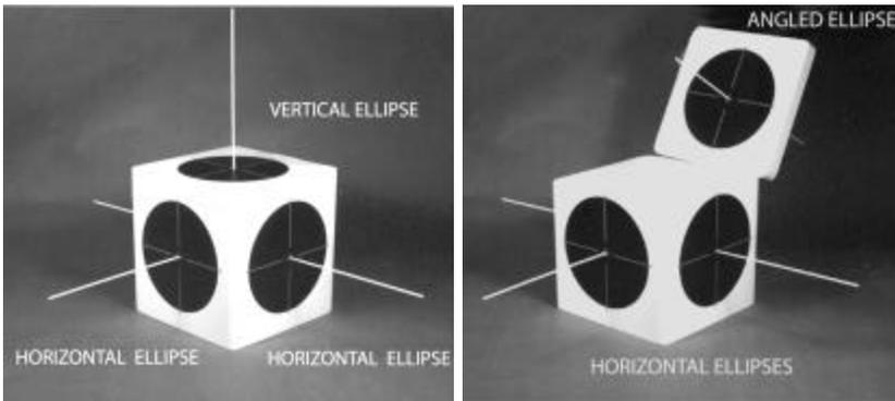
Obviously, the circles on the sides and top of the white cube appear as ellipses. Every ellipse has a major and minor axis, and the minor axis orientation is the key ingredient to drawing a visually correct circle (ellipse) in perspective.
