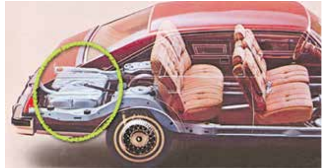
Through the 1960's, '70s and '80s, the fuel tank in most cars was located within the rear crush zone, exposing the fuel tank to being crushed punctured and ruptured in common rear-impact accidents.
