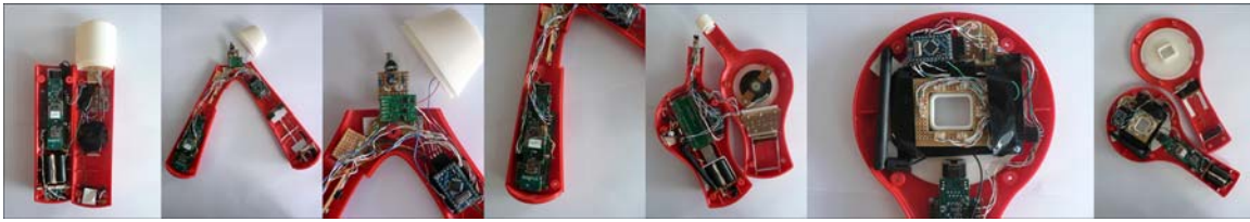
Each handheld device contains a full wireless computer + a combination of sensors
